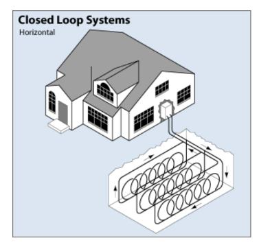
The geothermal heat pump system includes underground piping filled with liquid buried in shallow earth near the building. There is also a heat exchanger and the ductwork to connect it all together.
