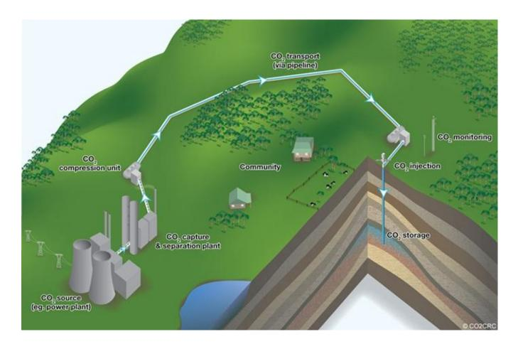
The power plant captures the carbon dioxide before it leaves the plant, then transports it to a site where they can inject it back into the ground.
