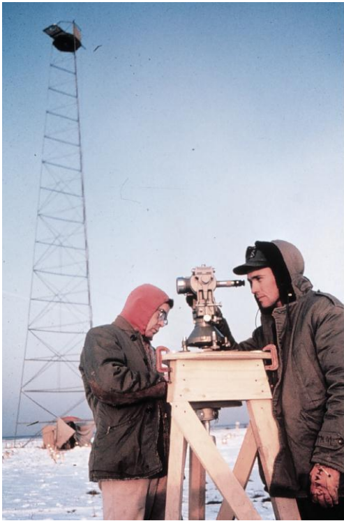
Ground-surveying techniques are conventional but precise for taking ground-based measurements.
