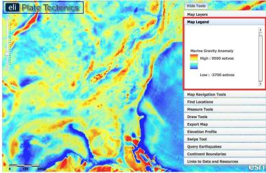
Because these different parts of the lithosphere have differing densities, the margin between them can be seen on a gravity anomaly map.
