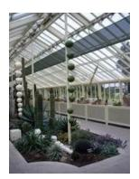
Heating Spaces: Greenhouses use passive solar heating but homes and other buildings can too. Glass windows are transparent to visible light, which warms in interior space. However, glass is opaque to infrared wavelengths given off by the interior, so the heat is trapped (thus the "greenhouse effect"). In warmer weather, an overhang can prevent sunlight from entering through the windows.
