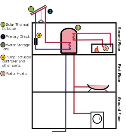
**2. Primary Circuit:** The solar collector and external part of the tank comprise the primary circuit.
