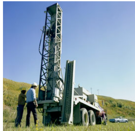
Operators Preparing a Hole for the Explosive Charges Used in Seismic Exploration
